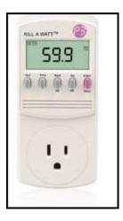
I measured 2.5 KWH (Kilowatt Hours) over a 24-hour period. This computes to less than \$10 per month for my entire PC setup. It surprised me to find out that one of my printers, an HP 6310 uses 9 watts when turned on and 6.5 watts by just being plugged in. Turning it off would save \$0.21 per month and unplugging it would save \$1 per month. Who would thought? The most frugal setup is to plug all equipment into a power strip and turn it off when not in use.
